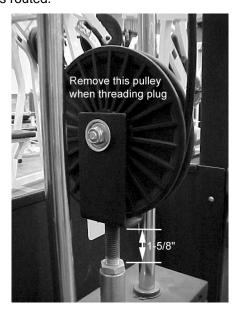
Figure 12. Bolt the floating pulley into the 190 lb weight stack (on cable crossover).
